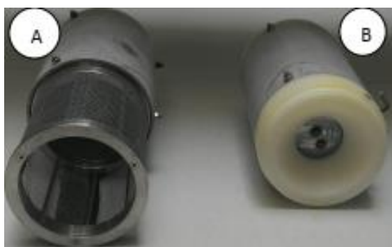
Fig 1: Device used to evaluate the repellent effect of essential oils: treatment chamber A and untreated chamber B.
