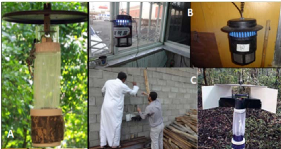
Fig 2: CDC miniature light (A), Black Hole (B) and Black light (C) traps.
