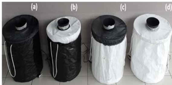
Fig 1: BGS traps with (a) a black cylindrical body and black nylon covering; BB, (b) a black cylindrical body and white nylon covering; BW (c) a white cylindrical body and black nylon covering; WB, and (d) a white cylindrical body and white nylon covering; WW.
